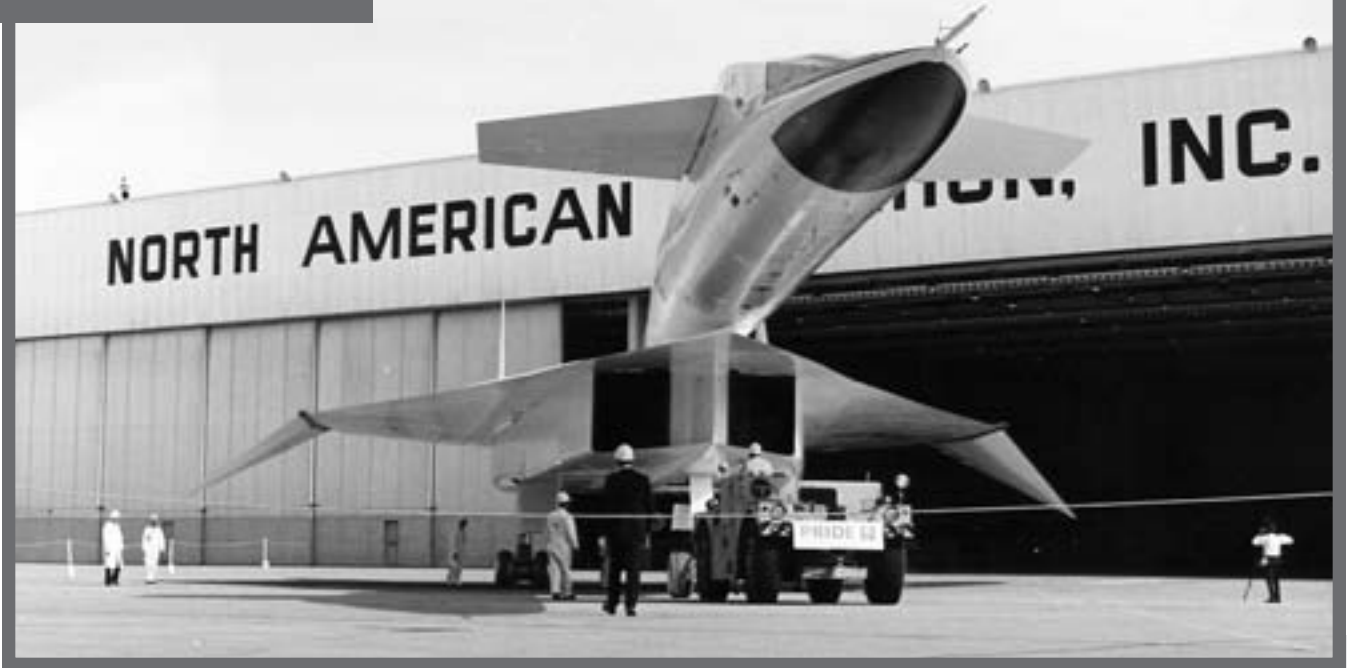
The No. 2 XB-70 was rolled out on 29 May 1965 at North American's Palmdale, California, facility. AV-2 was distinguishable from its sister ship by a black nose-chin radome and a more pronounced wingtip dihedral. (AFFTC Museum)
