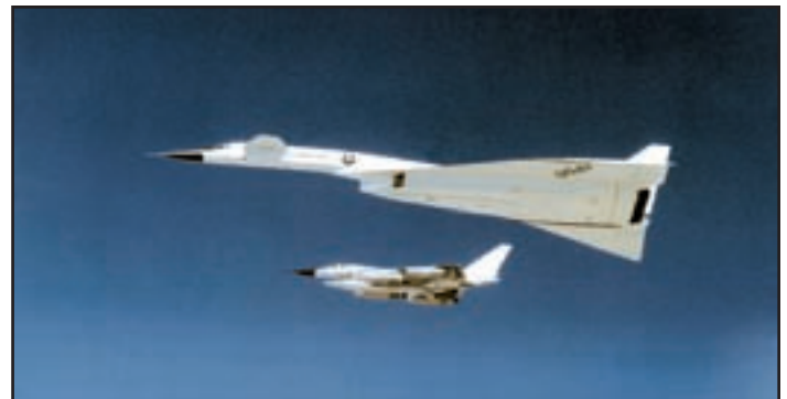
The Mach 2, delta-winged TB-58A served as pilot trainer and chase for the XB-70. (AFTTC History Office)
