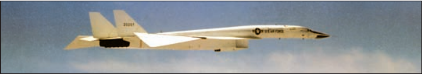
The XB-70 cruises over the clouds with wingtips down. AV-2 eventually demonstrated the ability to maintain Mach 3 speeds for more than 30 minutes. (AFTTC History Office)
