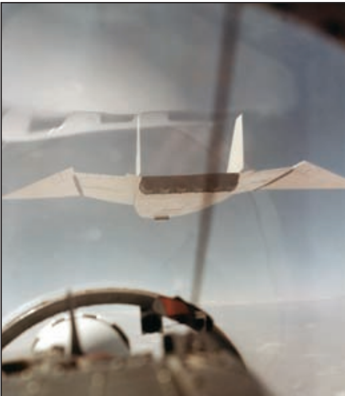
Seen from a chase plane, the XB-70 shows off its “six pack” of General Electric YJ93 afterburning turbojet engines, each of which generated 30,000 pounds of thrust. (AFTTC Museum)
