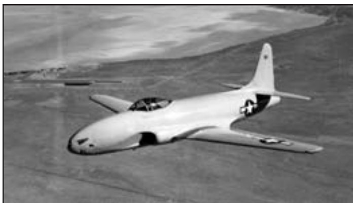
The first of two XP-80A preproduction prototypes, seen here over Muroc Flight Test Base, was known as the "Gray Ghost." It served as a testbed for a new engine and intake duct design improvements. (AFFTC History Office)
