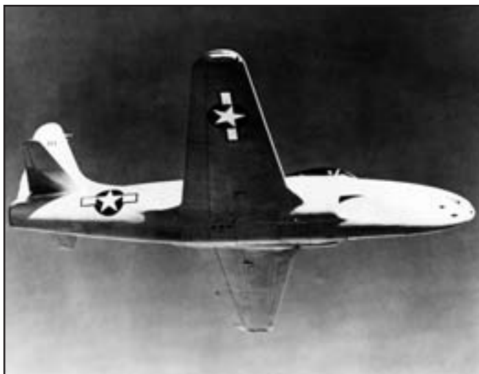
During a flight in the XP-80A to investigate engine intake-duct rumble, one of the jet's turbine wheels disintegrated, resulting in loss of the airplane. Tony LeVier bailed out at low altitude and survived with back injuries. (AFFTC History Office)
