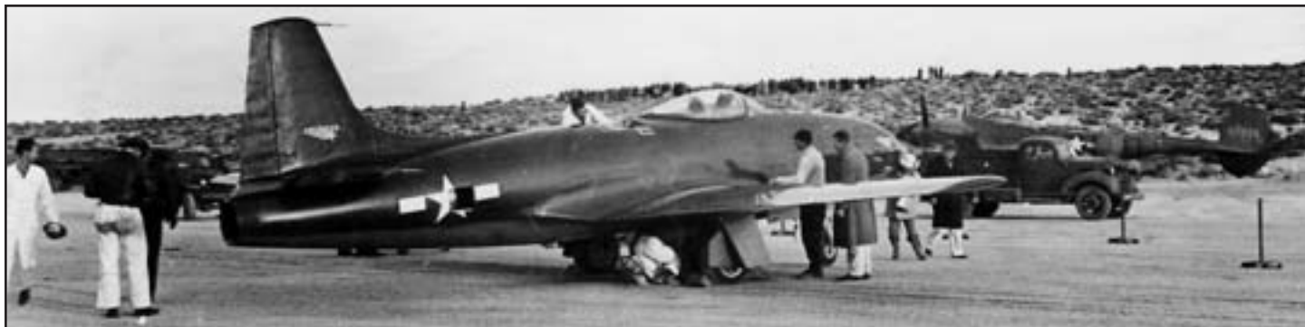
Lockheed chief test pilot Milo Burcham prepares to make the first flight in the XP-80 at the north end of Rogers Lake in 1943. Powered by a British Goblin engine, the jet achieved a speed of 547 mph in level flight. (AFFTC History Office)
