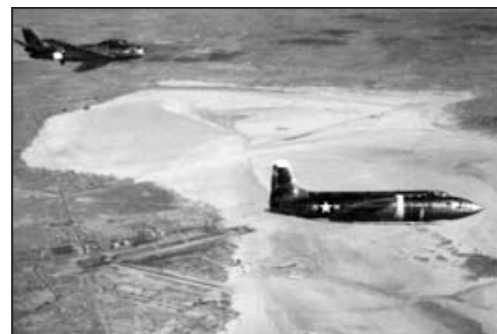
An F-86 chase plane accompanies the X-1A as it glides toward a lakebed landing at Edwards following engine shutdown. (NASA)
