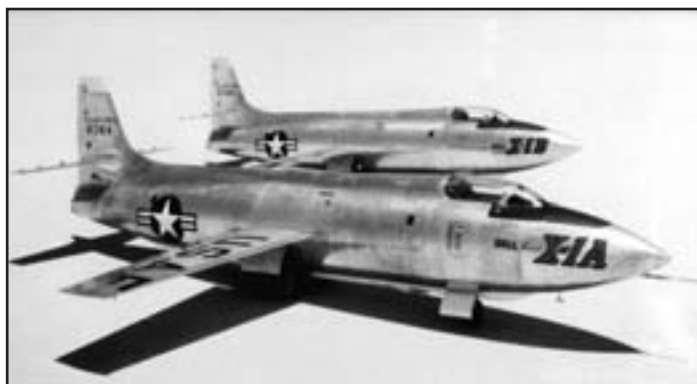
The X-1A and X-1B were slightly larger than their predecessors. New design features included an improved cockpit and increased fuel capacity. (AFFTC History Office)
