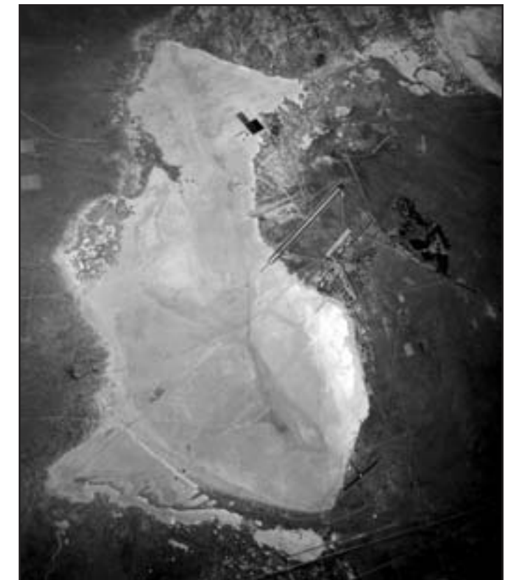
The parched bed of Rogers Lake provides 44 square miles of hard surface for aircraft operations. When dry, the clay can easily support the weight of the largest transport in the Air Force inventory. The lakebed has served as the landing site of space shuttles and numerous experimental planes. (NASA)
