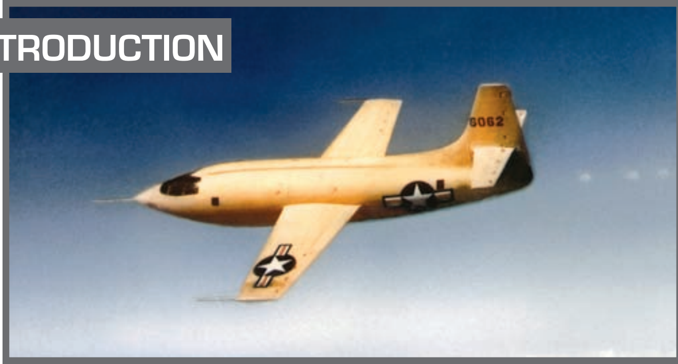
The Bell X-1, designed to mimic the shape of a .50-caliber projectile, was the first aircraft to explore the transonic region and break the “sound barrier.” (AFFTC History Office)
