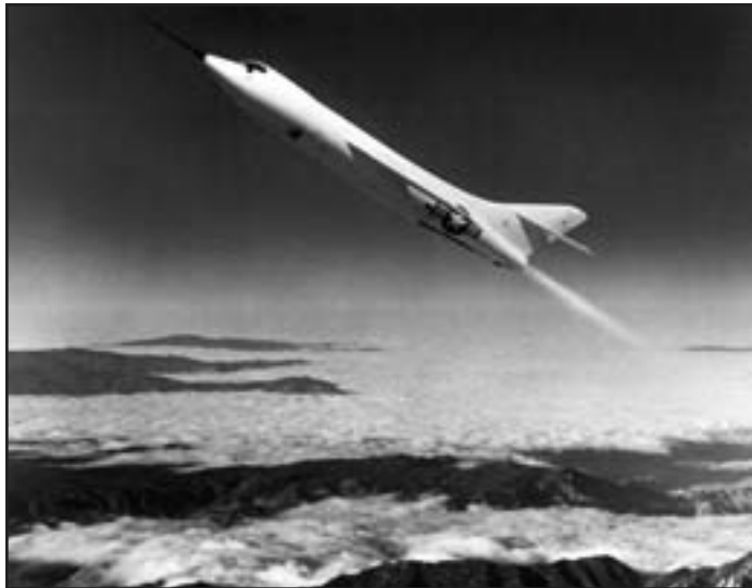
Although it did not carry an “X” designation, the jet-and-rocket powered Douglas D-558-II was a purely experimental design. It became the first manned aircraft to fly twice the speed of sound. (NASA)
