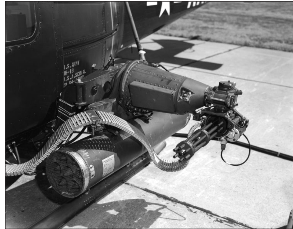
The UH-1C (S/N 64-14102) was a weapons training aircraft, seen here mounting the XM-21 system. Attached to the universal mount is an XM-157 rocket launcher with the M134 minigun mounted on a pylon extension. (U.S. Army)
