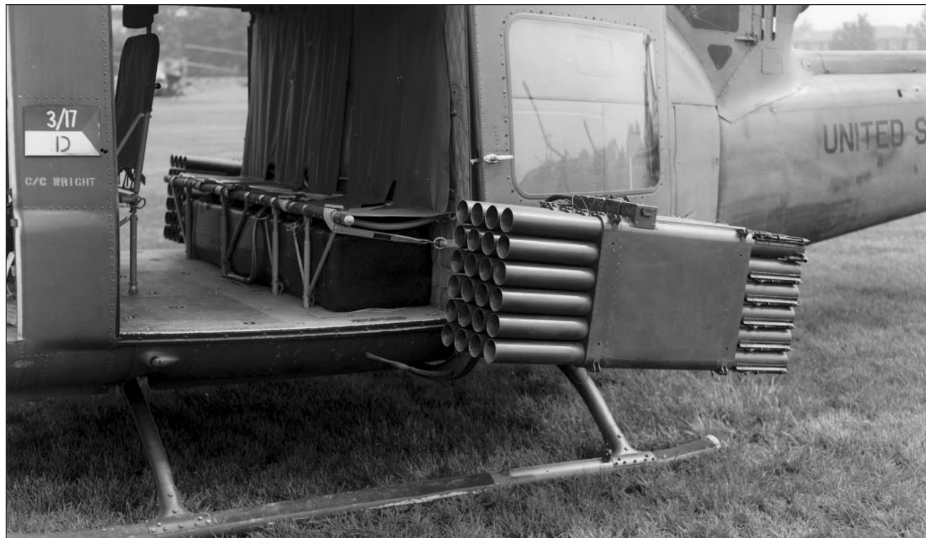
The 24-tube XM-3 was widely used during the early days of the Huey helicopter. It is seen here mounted to a UH-1B wearing markings of the Aerial Reconnaissance and Security Troop, D Troop, 3rd Squadron, 17th Cavalry at Fort Benning, Georgia, in 1963. An auxiliary fuel tank is under the troop seats, the red fabric of which was later changed to sage green. (U.S. Army)
