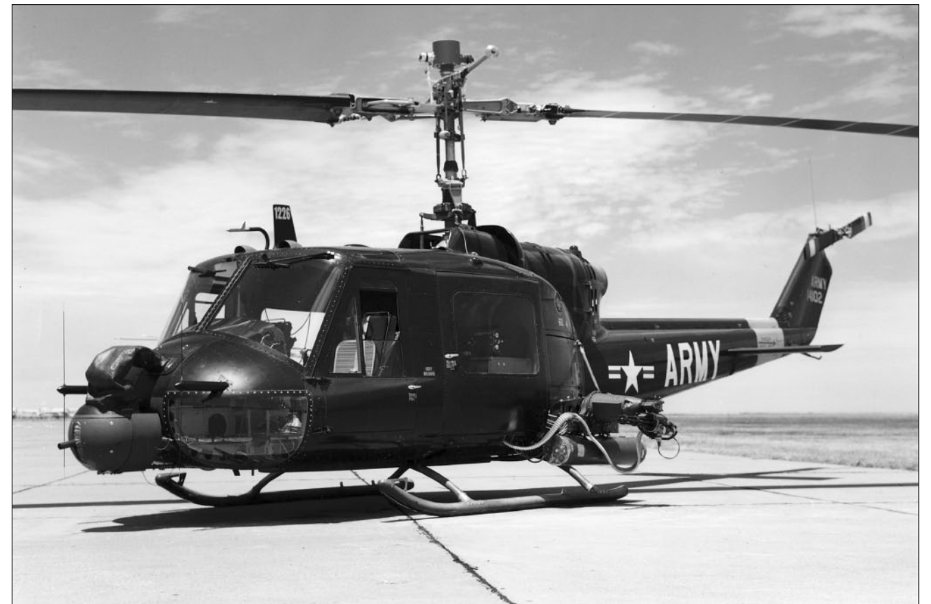
Outfitted with test instrumentation, Serial Number 64-14102, the second-built UH-1C, is armed with the XM-21 and XM-5 systems. This weapon combination was not used operationally since ammunition loads for both systems exceeded weight and space limitations. Later visible changes in the Charlie model line included a revised engine air intake unit, armored pilot seats, and relocation of the FM homing antennae on the nose. The aircraft's constructor number, 1226, is worn on the vertical blade-type VHF/UHF antenna. (U.S. Army)
