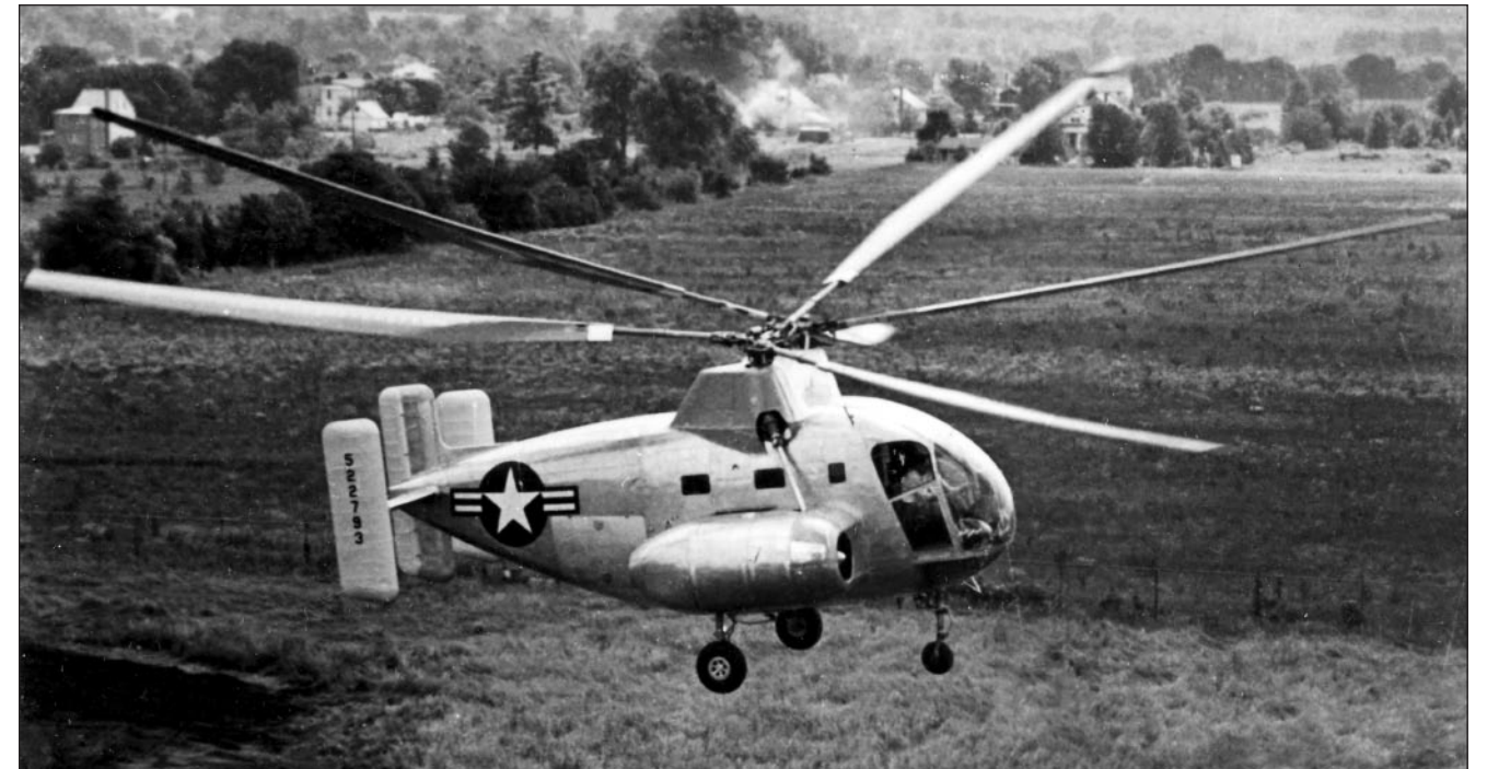
Kellett's final helicopter design for the Army was this XR-10. An enlarged version of the XR-8 able to carry six litters, it was powered by two 450-hp R-985-AN-5 engines. External engine mounting allowed full use of the cargo area. This example (S/N 45-22793) was one of two prototypes built before a production order for 10 machines was canceled. (Author's Collection)
