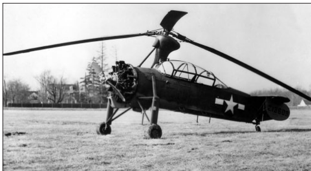
The Army's second rotorcraft was Kellett's KD-1 Autogiro, procured as the YG-1 (S/N 35-278). This aircraft, along with a YG-1A, crashed, leading to an order for seven YG-1Bs powered by 225-hp R-755-3 engines. The sustained power of an autogiro's rotor made it one step from being a helicopter. (Author's Collection)
