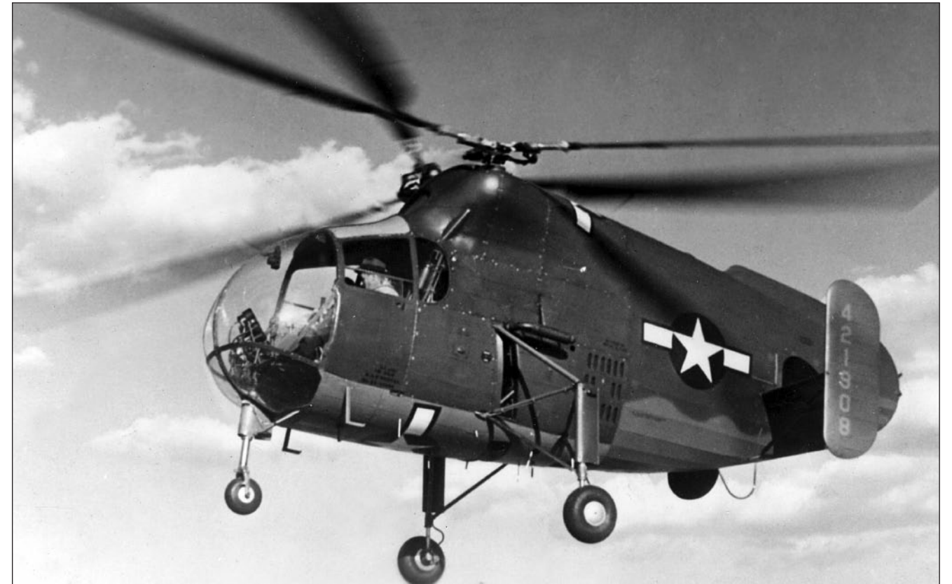
The beginning of the long line of Army helicopters continued with Kellett's XR-8, which followed Sikorsky's XR-4, -5, -6, and -7 models. The Kellett brothers favored German helicopter designer Flettner's intermeshing rotor, which ruled out the need for a tail rotor to counter torque. This aircraft (S/N 44-21908) was one of two prototypes built before rotor stability problems ended the program. (Author's Collection)
