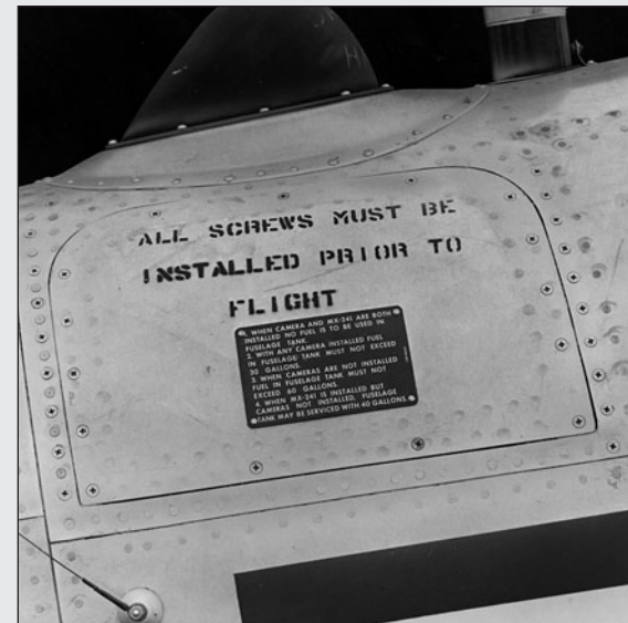
This large panel on the right side of the fuselage allowed access to the cameras and ADF. The placard notes that if cameras and MX-241 were installed, then the fuselage tank had to be empty.
