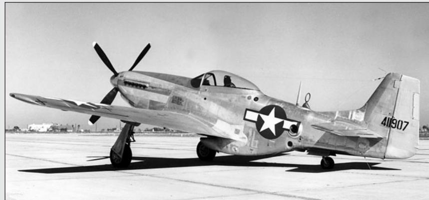
F-6K 44-11907 awaits delivery on the broad concrete ramp of the Dallas facility. Note how the national insignia wrapped around the camera port. Although difficult to see, the third camera port was located directly in front of the tail wheel doors.
