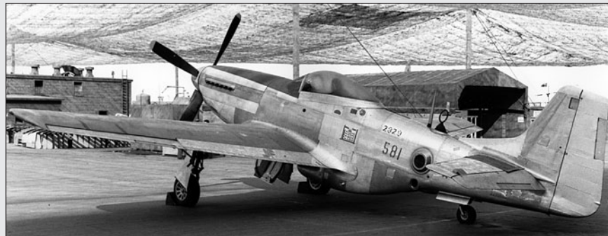
Parked under the camouflage netting at Inglewood (the more subdued light shows how different types of aluminum contrasted with each other). The aircraft's wing was still in primer finish and national markings and serial had yet to be applied. The Automatic Direction Finder (ADF) was directly above the camera port. ADF is a radio receiver equipped with direction-sensing antenna used to take bearings on a radio transmission.
