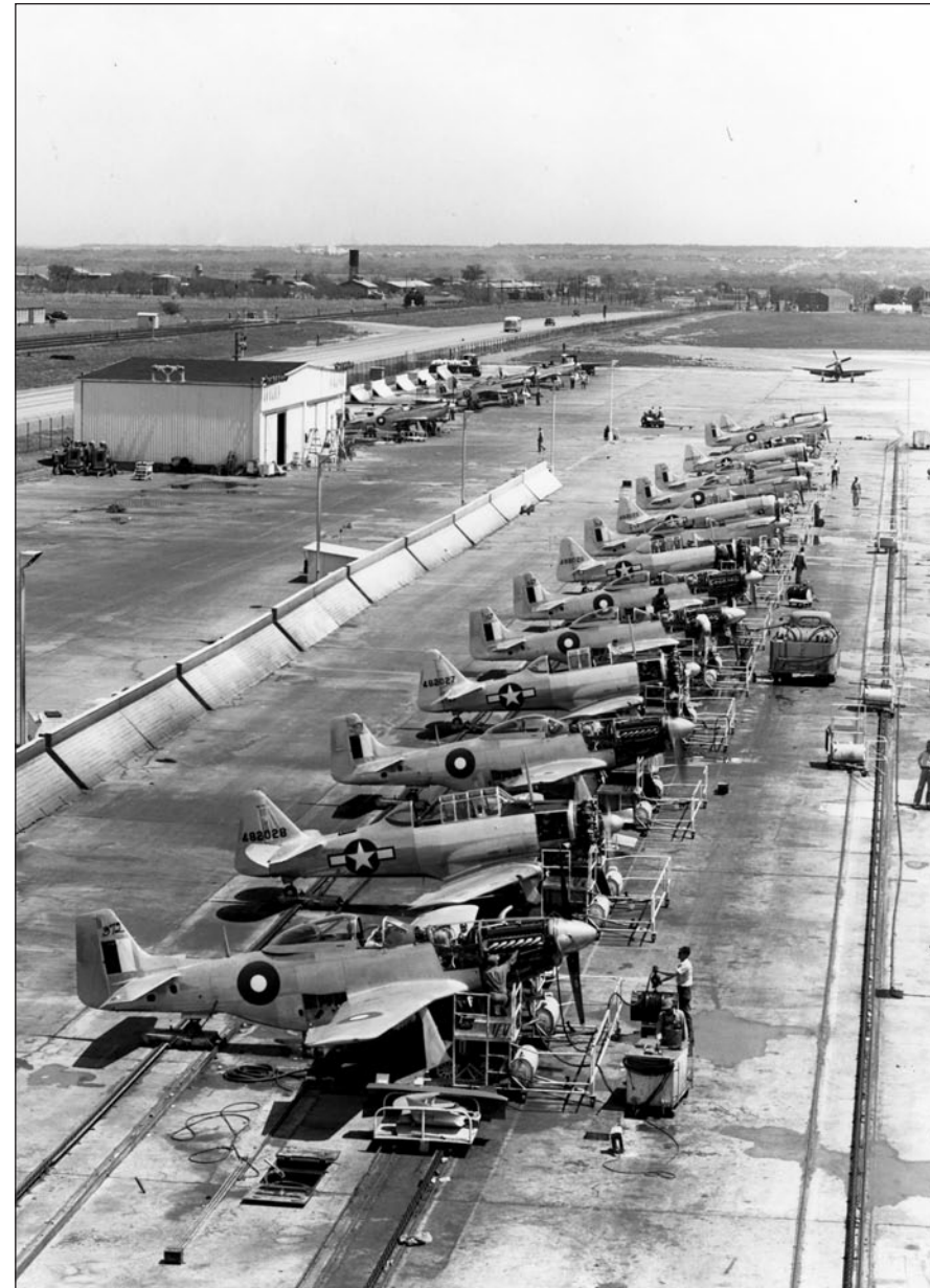
High-angle view of the engine test area shows the railings to which the aircraft were attached. With the end of the war, the huge plant became almost a ghost town.
