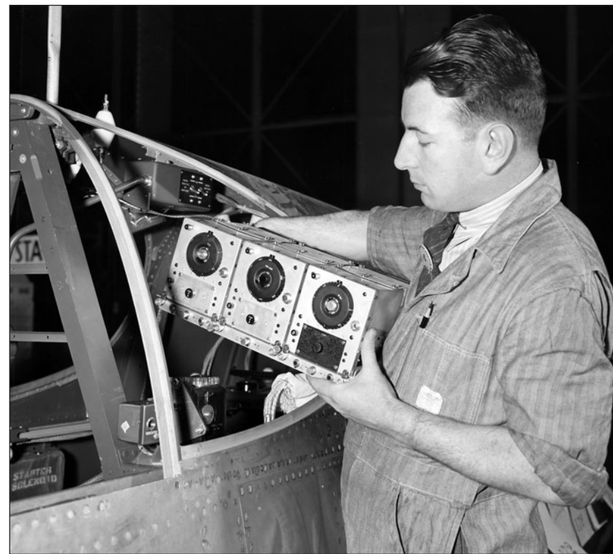
At each step of the production line, components were added to the Mustang in an orderly fashion. In this case, a worker installs the SCR-274 command radio behind the P-51A pilot's position. This radio was the main communication between the pilot, ground bases, and other aircraft. The substantial rollover structure immediately forward of the radio compartment would save many pilots during takeoff and landing accidents.
