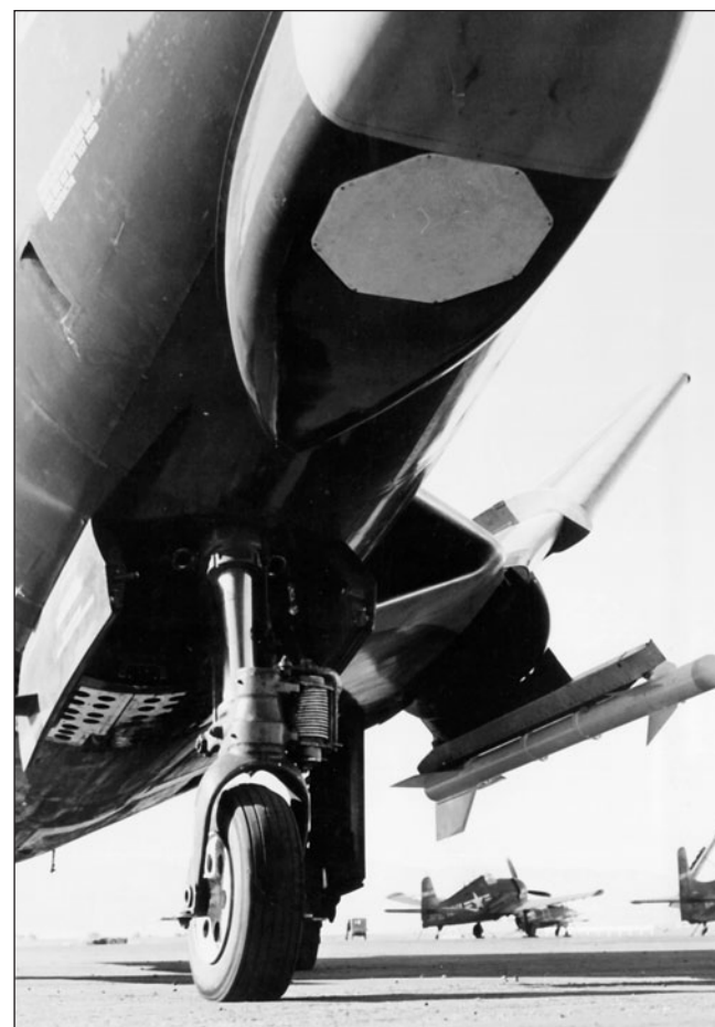
An excellent view of the under-nose fairing that houses the ARA-25 can be seen on this F9F-8. Note the Sidewinders on the wings. (National Archives)
