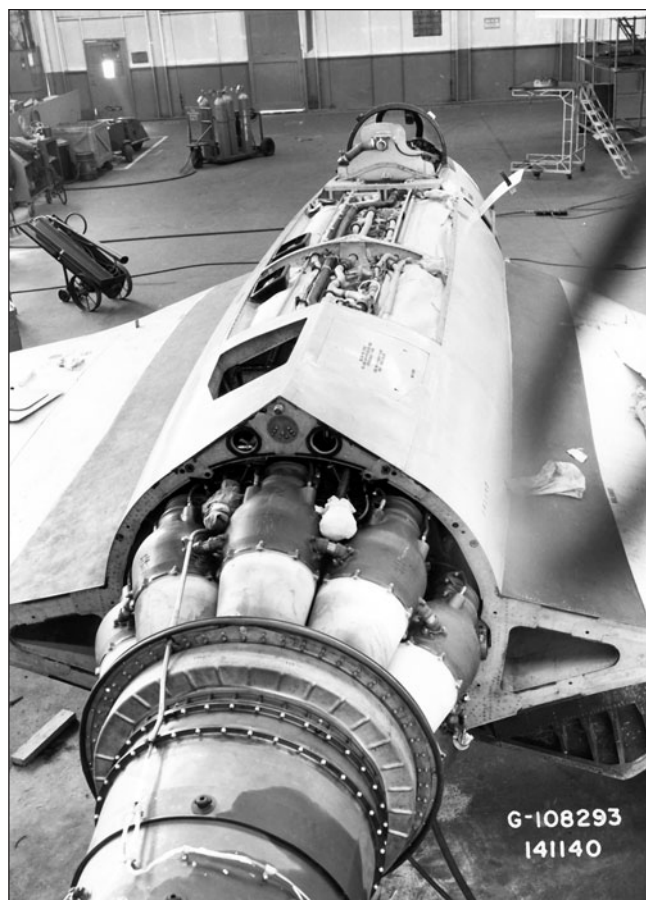
With its aft section removed, the engine of this Cougar is visible, as are the tops of the fuel cells. One of the "blow-in" engine air intakes is also open. (Jim Sullivan Collection)
