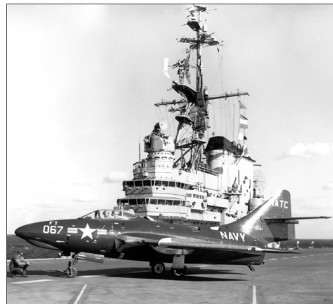
BuNo 131067 undergoes carrier suitability trials aboard USS Coral Sea (CVB-43). The "FT" on the nose denotes a NATC Flight Test Division aircraft. The pilot is about to move onto one of the forward catapults. (Jim Sullivan Collection)
