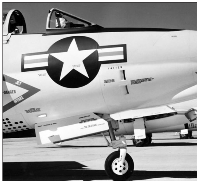
The forward section of the F9F-8 shows the extended nose and underside fairing for the jet's ARA-25 radar. This Cougar is painted in the modern gull gray with white underside, which replaced the earlier glossy sea blue. (Jim Sullivan Collection)
