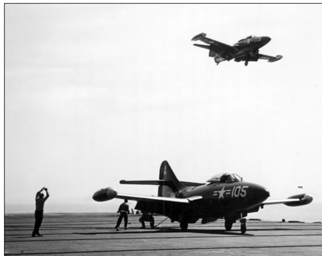
An F9F-2 Panther is removed from the arresting gear while another is waived off. Visible as a speck in the background is a third Panther beginning its roll into the groove as it prepares for final approach. (Bert Kinzey)
