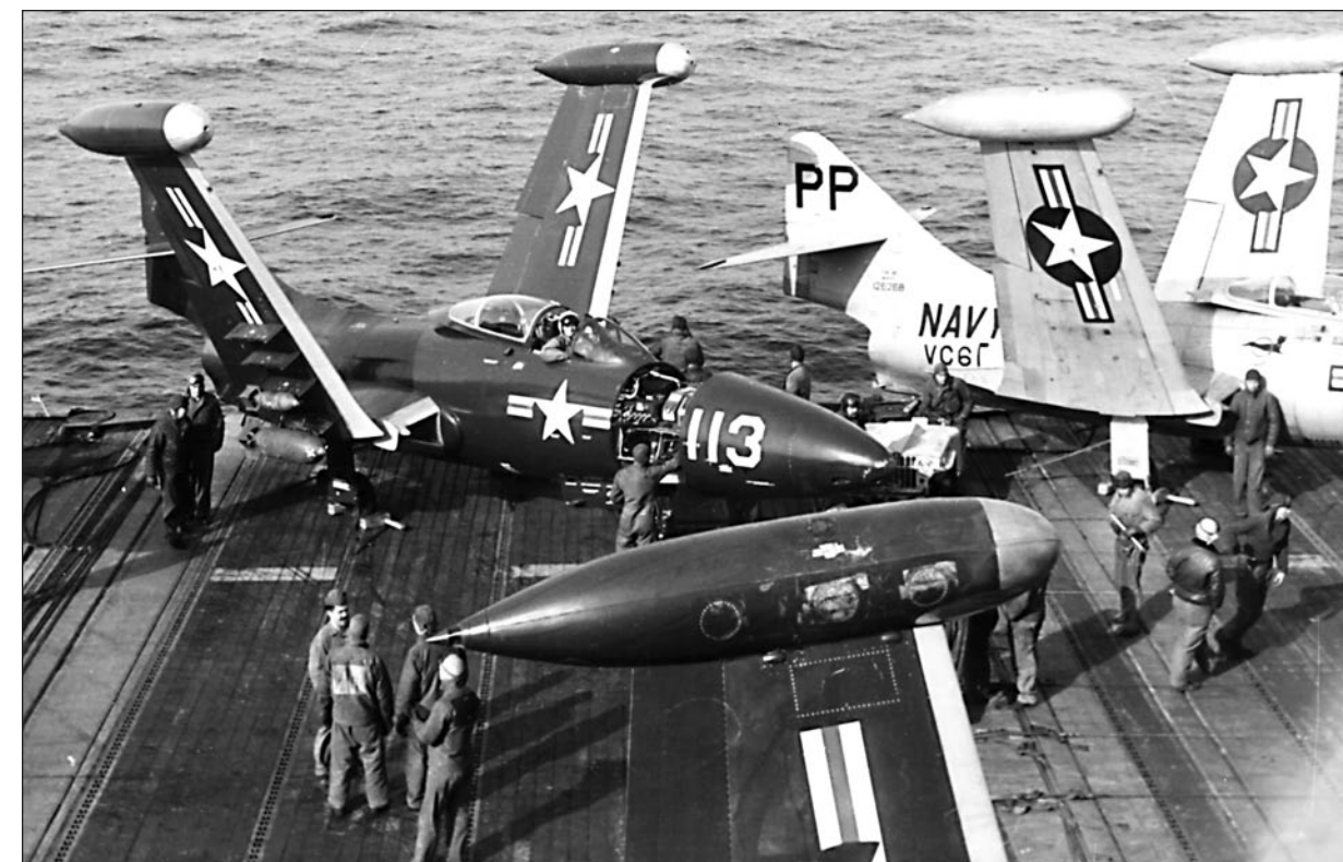
A VF-51 F9F-2 and VC-61 F9F-2P are readied for missions. The crew appears to be working on the Panther's guns. (Steve Ginter)
