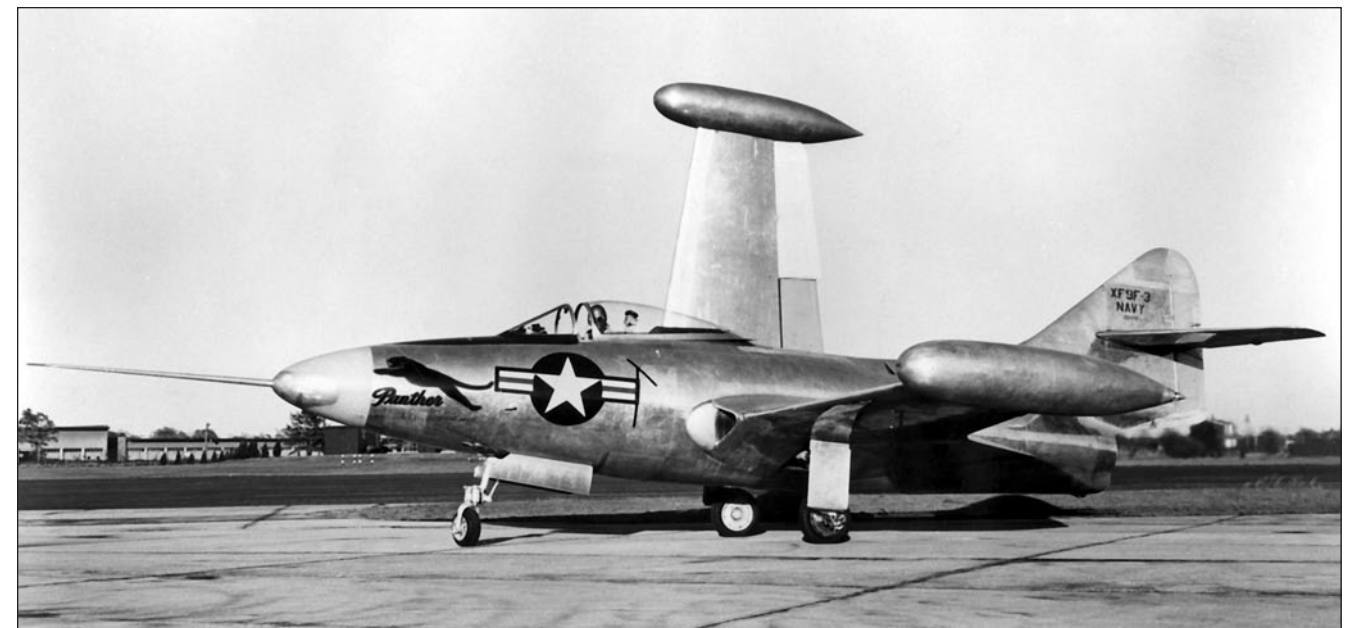
This picture shows the XF9F-3 at Bethpage in an odd configuration with one wing folded and the other in its proper inflight position. Note right aileron fully deflected upward. (Northrop Grumman History Center)
