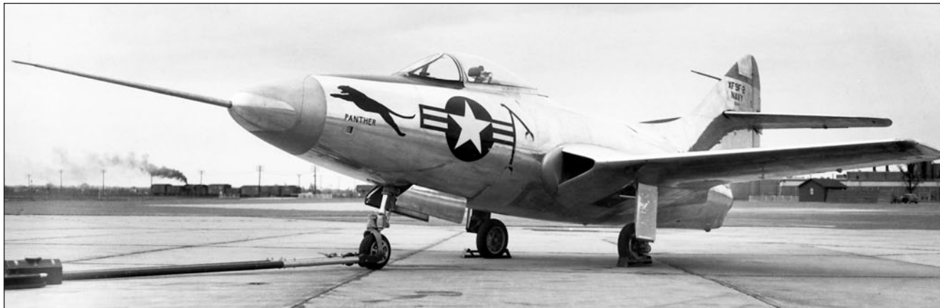
Now sporting a snazzy black-panther nose art insignia, an instrumented XF9F-2 awaits flight testing at Grumman's Bethpage plant. Note data booms mounted on both the nose and tailfin of the airplane. (Northrop Grumman History Center)
