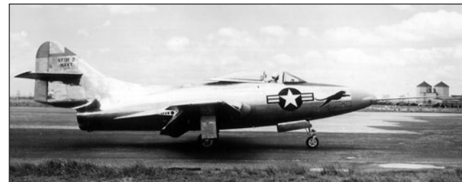
The second XF9F-2 prototype, BuNo 122477, is shown here on the runway at Bethpage, with instrumentation affixed to the nose and the black-panther insignia. (Northrop Grumman History Center)
