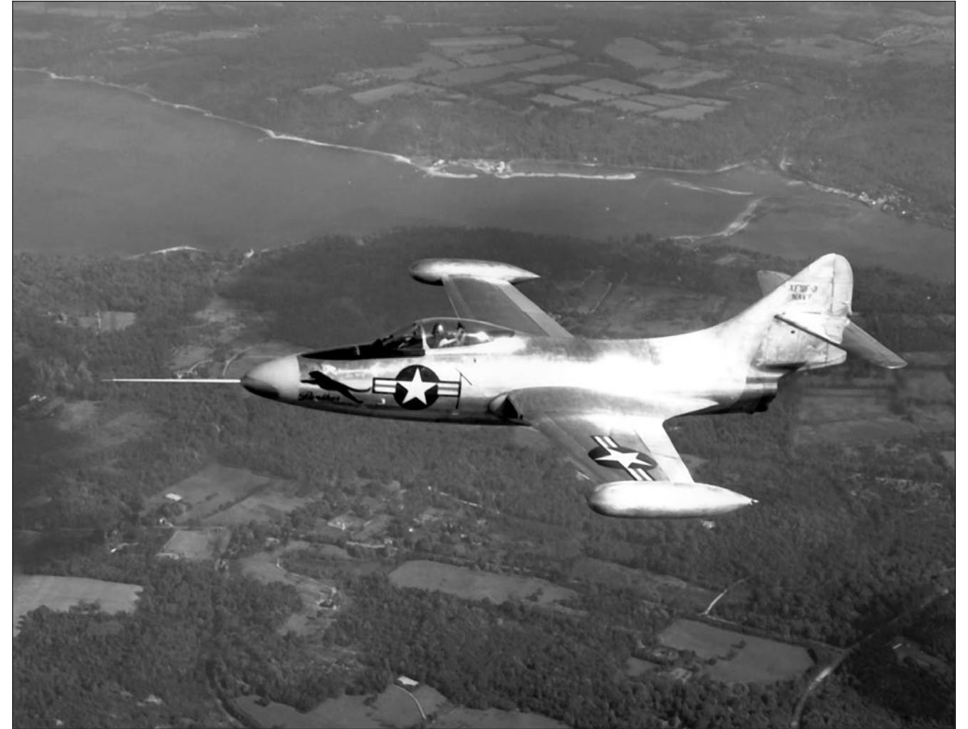
An excellent view of a highly polished XF9F-3 in flight sometime during 1948, with wingtip tanks installed. (Northrop Grumman History Center)
