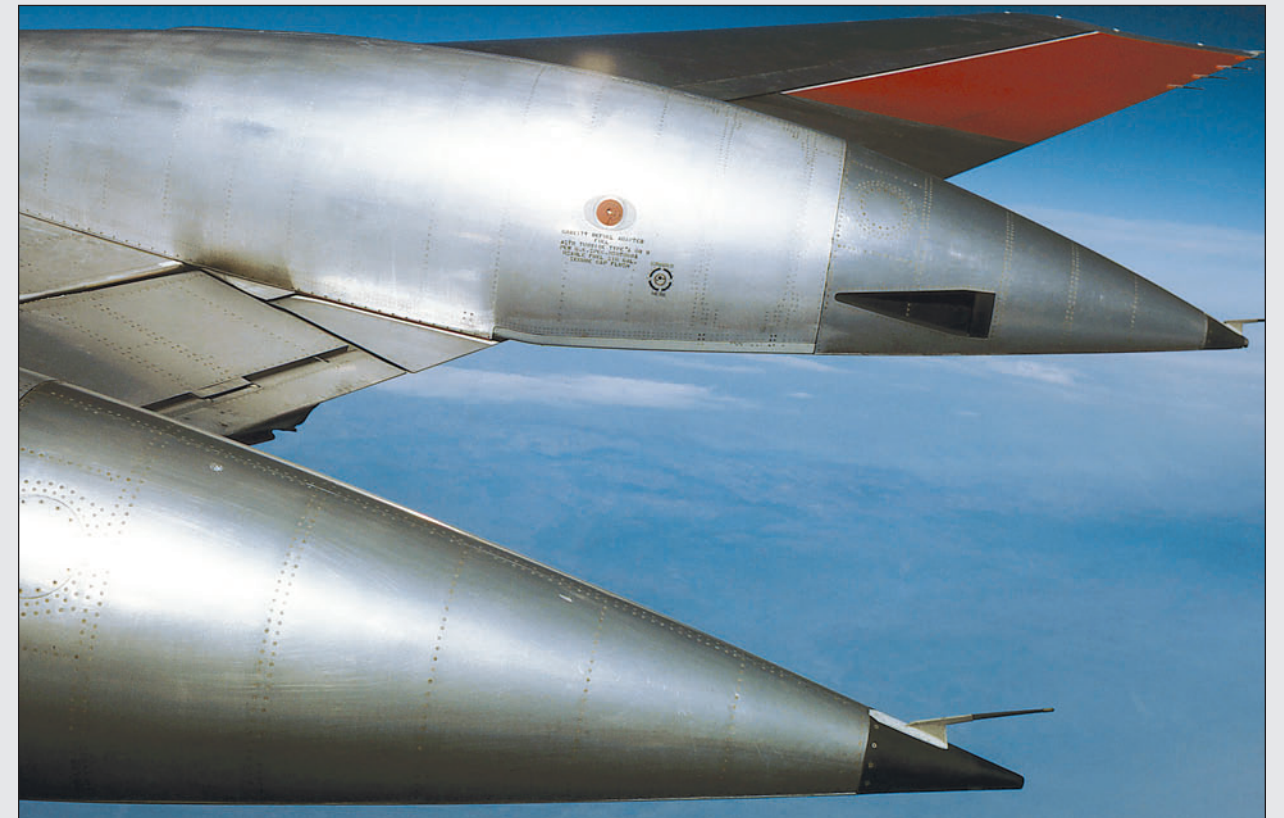
The 990 was the only commercial jetliner to utilize anti-shock bodies on the trailing edges of its ultra-thin wings. Added to take a continuous airflow over the upper wing surface, they lessened or delayed the shockwave that increased drag at speeds above Mach .80. The pods served as additional fuel tanks in all but the aft sections and also contained discharge nozzles for fuel jettisoning. (Jon Proctor Collection)
