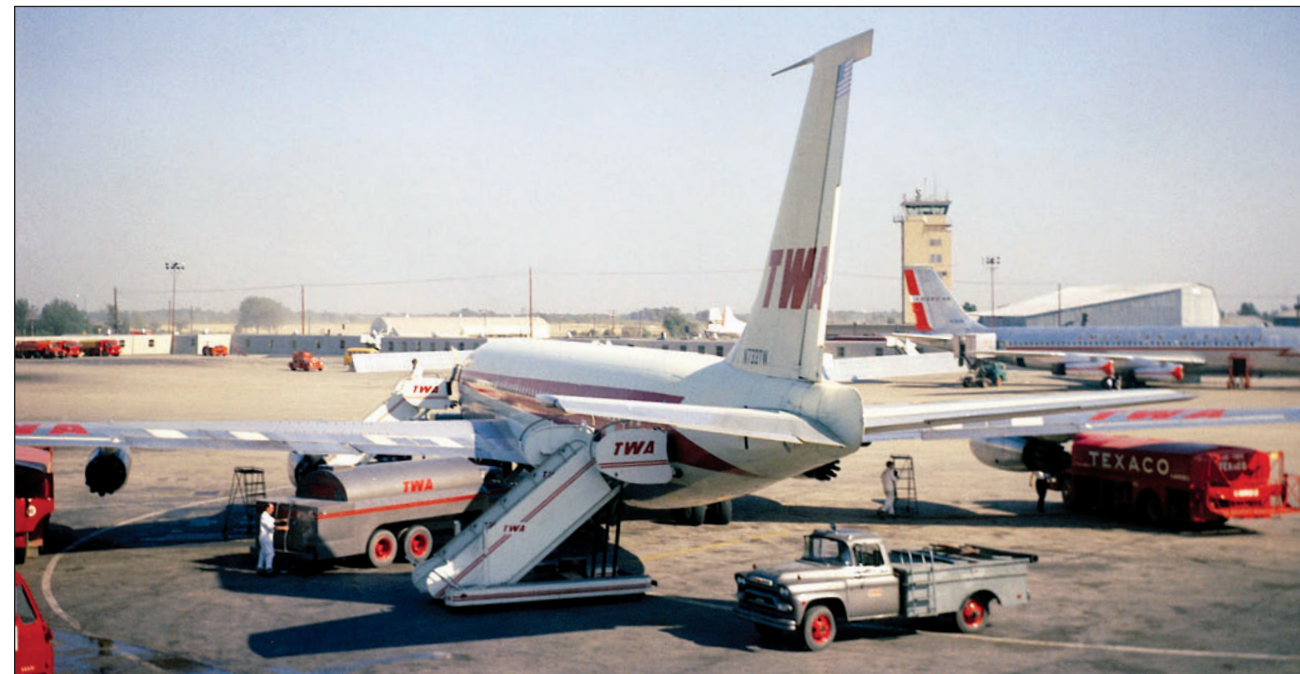
Graphically demonstrating the transition period from props to jets, we see a TWA Boeing 707 at Chicago-O'Hare surrounded by a sea of ground equipment as listed on page 99. Manually pushed boarding stairs exposed to the elements soon gave way to fully enclosed and extendable jet bridges attached directly to the terminal building. (Jon Proctor)
