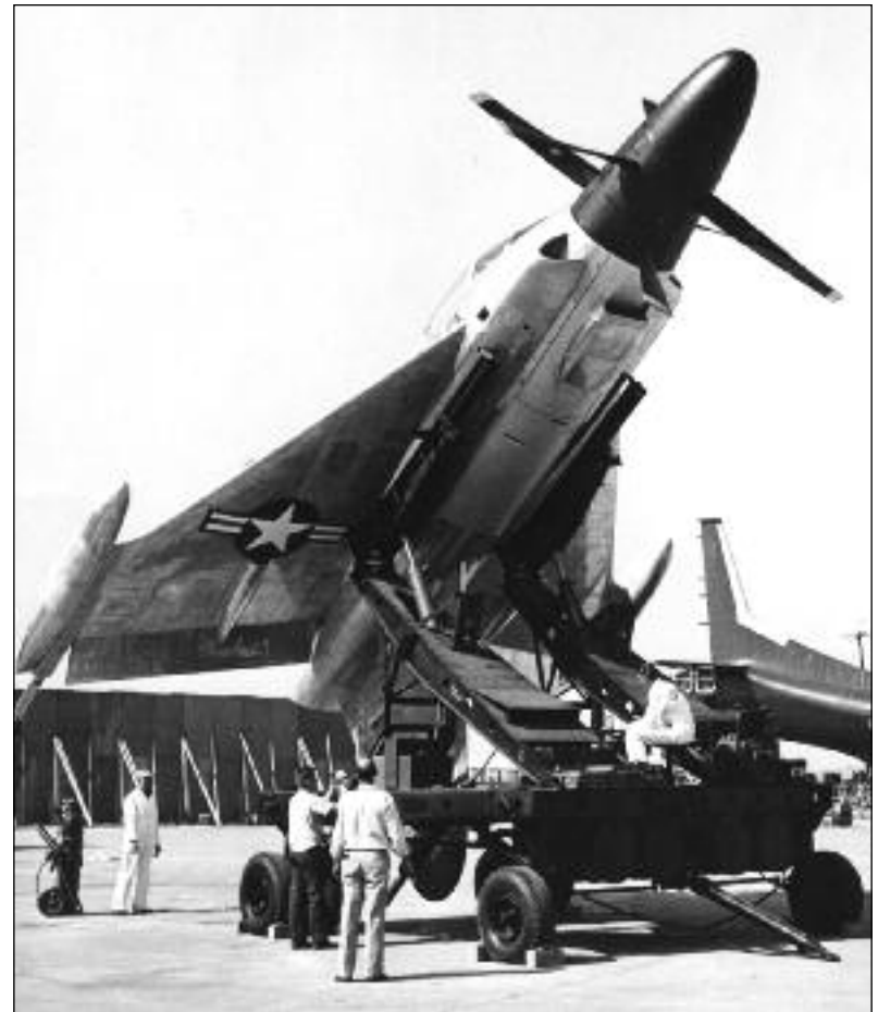
Unlike the Lockheed XFY-1, the Convair XFY-1 was not configured for horizontal take-off, so in order to transport it horizontally on the ground it was mounted to this specially designed hydraulic apparatus and slowly lowered from vertical. This trailer was used to transport the Pogo between San Diego and Brown Field Auxiliary Naval Air Station. (Convair via Author’s collection)
