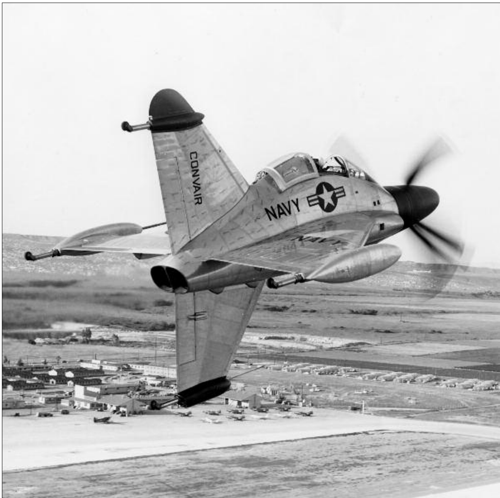
With his cockpit canopy in the open position, Skeets Coleman thunders over Brown Field Auxiliary Naval Air Station after having taken off vertically and converted to horizontal flight in the XFV-1. (Convair via Author's collection)
