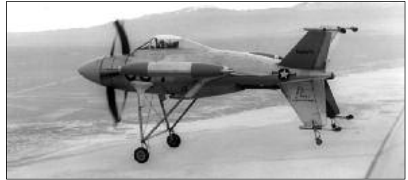
The Lockheed XFY-1 in horizontal flight with the apparatus that was used for horizontal take-offs. The Lockheed aircraft was able to convert to vertical flight after a horizontal takeoff, but it never took off vertically. (Author’s collection)
