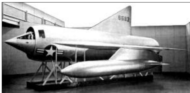
Here, the XP-92 is dwarfed by its own auxiliary fuel tanks. Convair proposed this arrangement for the early part of a mission when a great deal of fuel would be used, pushing the interceptor to high altitudes at great speed. (Convair via Robert Bradley)
