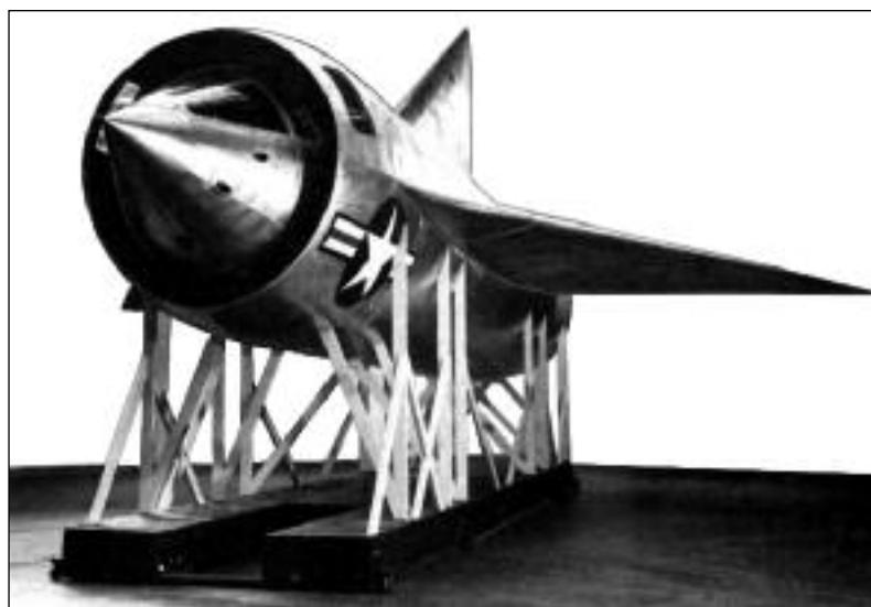
As shown in the 1948 mock-up, this proposed XP-92 located the cockpit within the spike in the center main ducted-rocket intake! (Convair via Robert Bradley)
