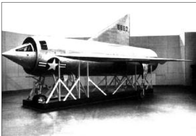
By late April 1948, when the U.S. Air Force inspected this mock-up in San Diego, the XP-92 design had evolved from swept wings to delta wings. (Convair via Robert Bradley)
