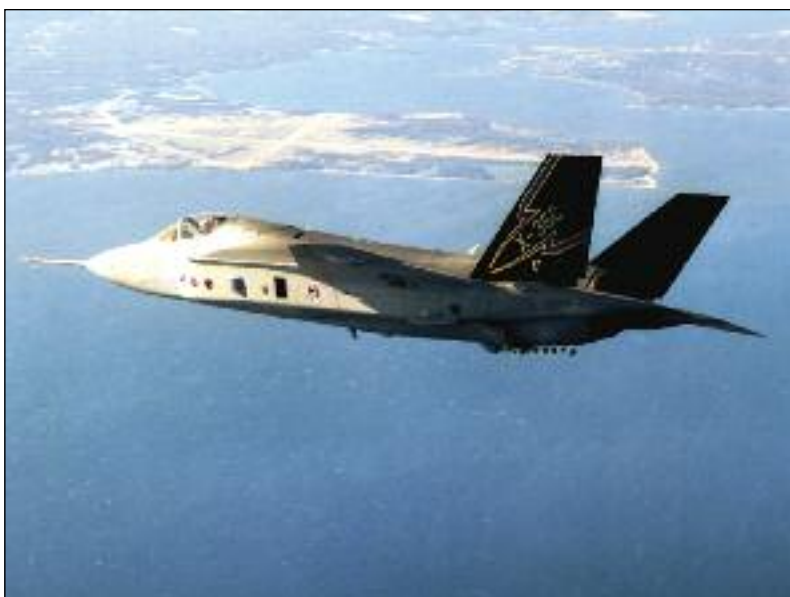
The naval variant of the Lockheed Martin JSF, the X-35C, was only used for handling quality and performance testing, not actual arrested landings. The major external difference besides the tailhook was a larger wing. It is shown here arriving at NAS Patuxent River in February 2001 for evaluation. (U.S. Navy 010210-N-0000P-001)
