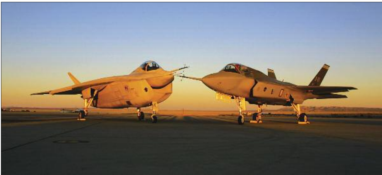
The two contenders for the JSF program, the Boeing X-32 on the left and the Lockheed Martin X-35 on the right, are posed together on the ramp at Edwards Air Force Base. The Boeing has the more innovative aerodynamic configuration. The Lockheed vertical takeoff and landing propulsion concept incorporating a lift fan is high risk but potentially provides more thrust in VTOL mode than simply diverting the engine exhaust. (Author's collection)
