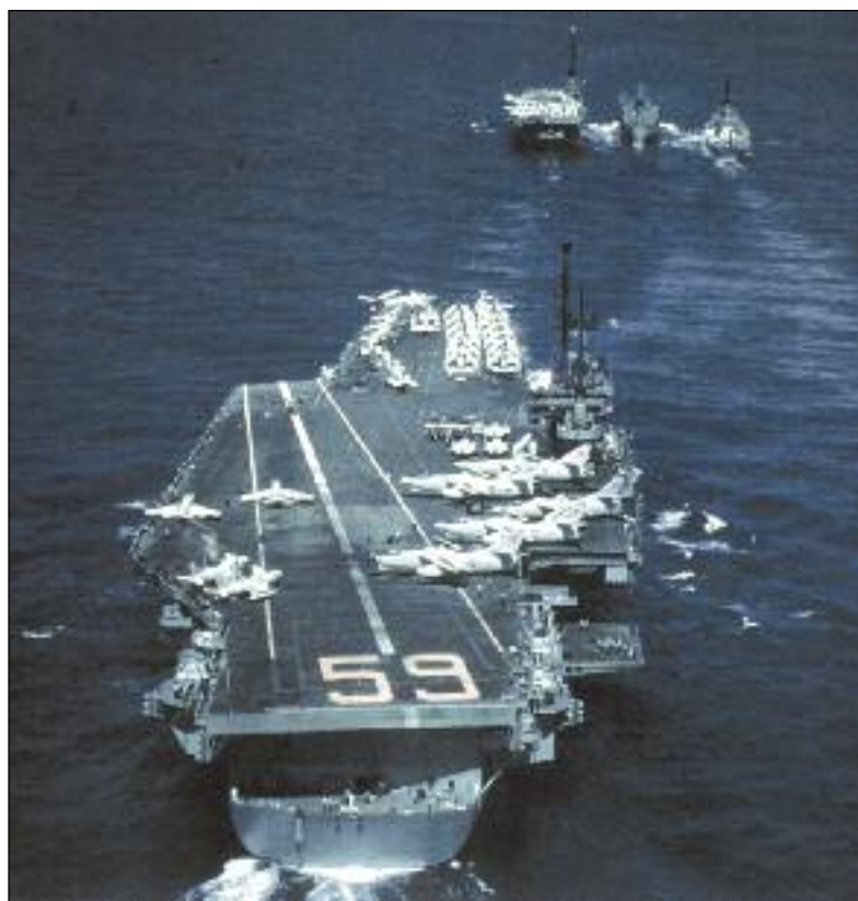
The realization of the Navy's late 1940s plan for a super carrier and a long-range atomic bomber are depicted here. Forrestal's first full deployment was made to the Mediterranean from January to July 1957. The air group included F3H-2Ns and FJ-3Ms for fighters and AD-6s, F9F-8Bs, and the A3D-1s for attack. Seven A3D-1s are on deck in this picture with FJ-3s on the axial-deck catapults standing ready. (National Archives 80-GK-22688)
