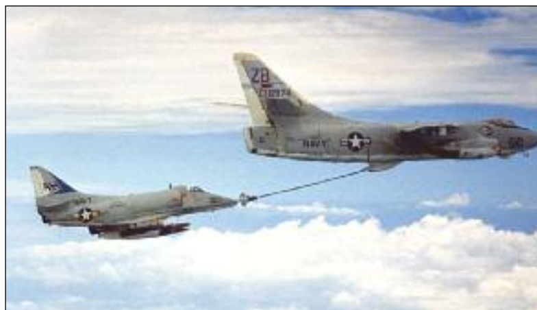
The A3D filled a vital supporting role as a tanker for fighters and bombers prior to ingress and after egress on strike missions in Vietnam. The bombardier/navigator has uncovered the periscope to view the proceedings. (Robert L. Lawson collection)
