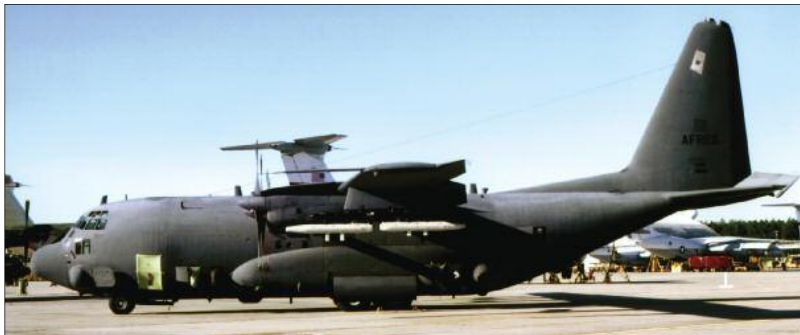
The AC-130A, S/N 54-1630, at Warner Robins AFB in October 1979. The AN/ALQ-87 ECM pods, seen in white, were mounted in pairs on underwing mounts. (R. Ray Leader via Stephen Miller)
