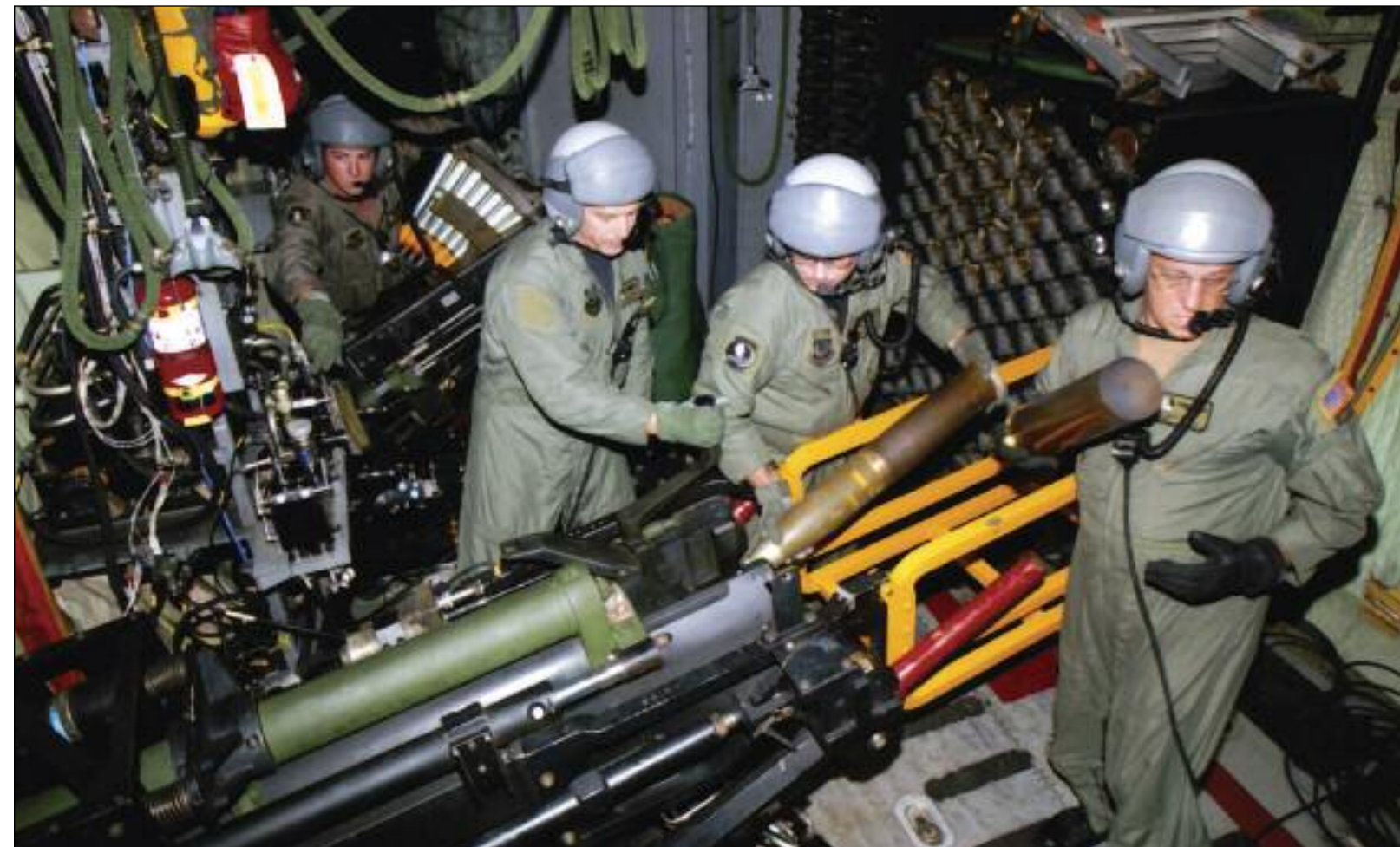
In the back of the AC-130U, three gunners operate the 105mm Howitzer, and one operates the 40mm Bofors cannon. The ammunition racks for both weapons are against the opposite side of the fuselage. (U.S. Air Force)
