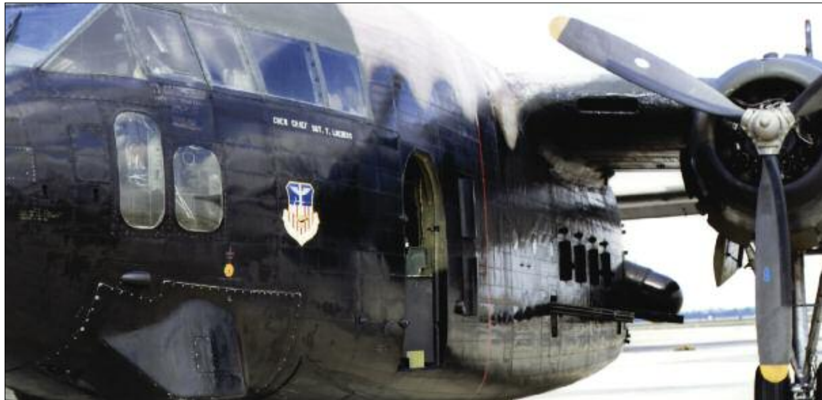
The added FLIR and 20mm cannons gave the Stinger a capability far superior to that of the Shadow in the search and destroy role. An armor panel covered the lower half of the forward doorway to protect the night observation sight operator. Two smoke-clearing air scoops immediately rearward of the doorway are closed. On the forward fuselage of S/N 52-5910 is the emblem of the 1st SOW. On some AC-119s, the two lower cockpit windows on both sides of the fuselage were painted over with black. (Stephen Miller)
