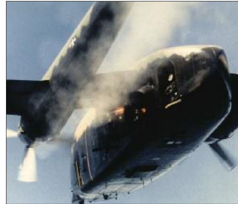
This impressive view of a Stinger firing one of its four miniguns illustrates the importance of wind spoilers used to direct gun smoke and gasses into the slipstream. (U.S. Air Force)
