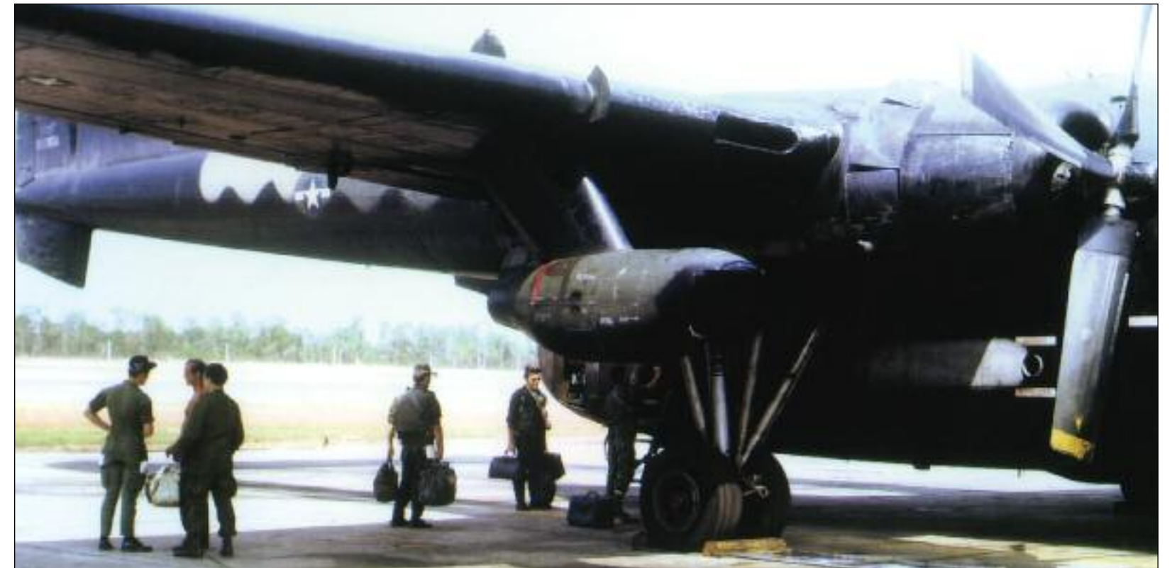
The crew of 53-3154 prepares for a mission from Nakhon Phanom RTAFB in 1971. Stingers were regular residents of NKP, flying interdiction missions in Laos. Heavy exhaust from the gas turbine stains the aircraft's mid-fuselage. (Tony Bautz)
