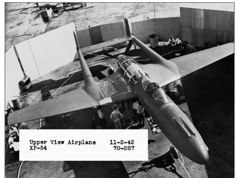
The XP-54 in a secure final assembly and checkout enclosure at the Vultee facility in Downey, California. The large size of the XP-54 is evident when compared to the mechanics working around the aircraft. Note the canopy enclosure has not been installed. (Convair)
