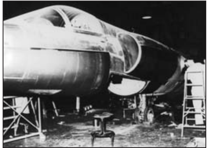
In 1957, Article 341 was partially coated with radar-absorbent materials. Because the coating added a great deal of excess drag, the airplane was dubbed a "Dirty Bird." (Central Intelligence Agency)
