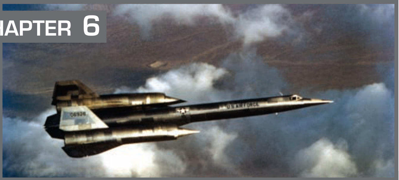
The third A-12, known as Article 123, served as a testbed for inertial navigation system and camera testing. It was the first Oxcart airframe to crash. (Lockheed via Jim Goodall)
