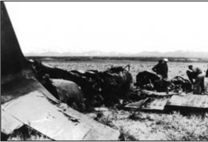
Lockheed personnel examine the wreckage of Article 341 in central Nevada. Engine overheating resulting from application of radar-absorbent material began a chain of events that culminated in loss of the airplane and pilot. (Central Intelligence Agency)
