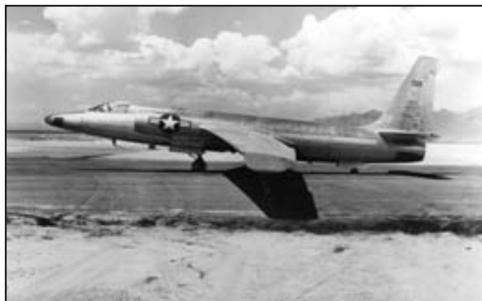
Lockheed’s U-2 prototype, known as Article 341, was designed to be lightweight and aerodynamically clean in order to facilitate flight at high altitudes. The original configuration was not optimized to avoid radar detection. (Lockheed Martin)
