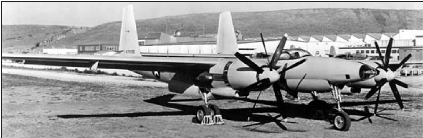
Parked at Culver City, the XF-11 shows off its 101-foot wingspan. The relatively small fuselage made the airplane appear deceptively small while it was, in fact, quite large for its time. (AFFTC Museum)
