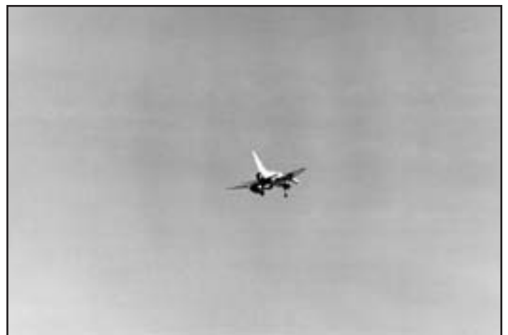
The second ZEL F-100 flight, on 11 April 1958, began with a successful launch. At booster burnout the airplane was traveling 300 mph at an altitude of about 250 feet. Under normal circumstances the booster would separate at this point, but in this case it remained attached to the F-100, making it impossible for the pilot to land safely. (AFFTC History Office)
