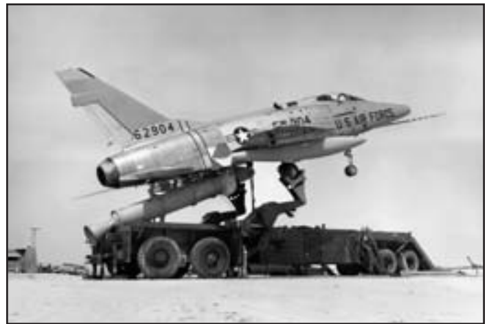
The ZEL F-100 carried a 275-gallon fuel tank on the right wing. This offset the weight of the weapon on the opposite wing and simulated the planned operational configuration. Had nuclear-armed ZEL fighters been launched in the event of all-out war, it was expected to be a one-way mission. (AFFTC History Office)
