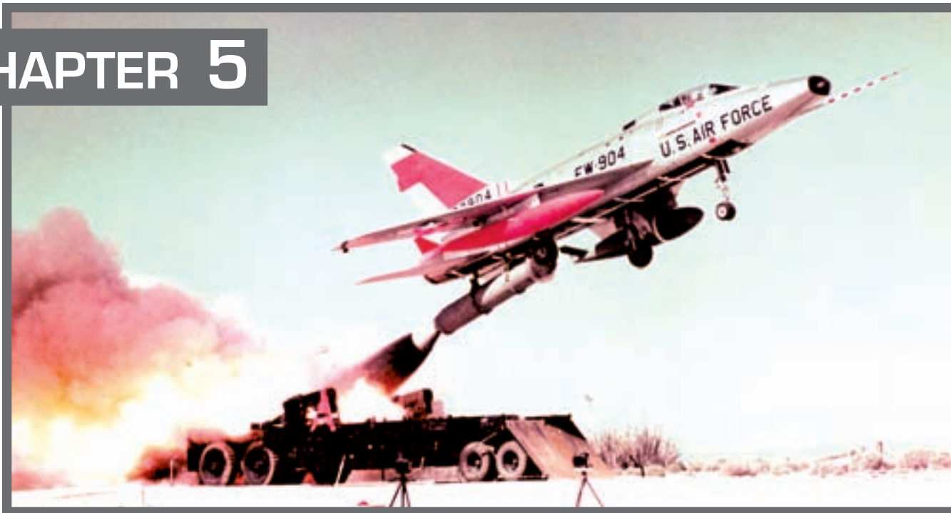
A Rocketdyne XM-34 booster generated 132,000 pounds of thrust for four seconds to loft the F-100 into the sky. The “takeoff run” amounted to three-eighths of an inch, making this one the world’s shortest runway. (U.S. Air Force)
