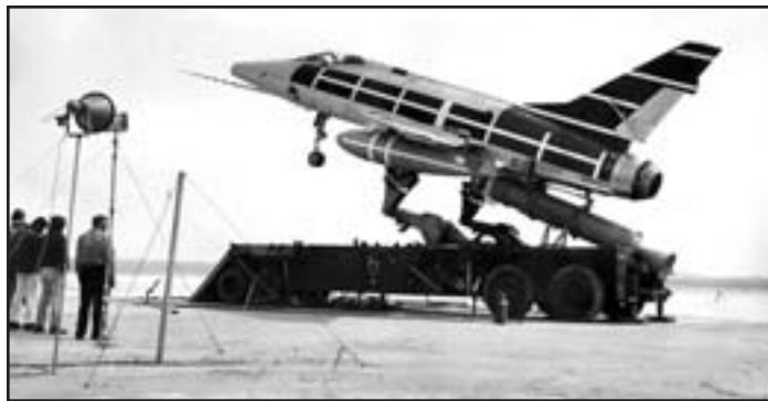
The Zero-length Launch, or ZEL, F-100 was equipped with a solid-propellant rocket booster and launched from a mobile platform. The airplane carried a T-63 (simulated Mk.7 nuclear weapon) on the left wing. The black-and-white grid on the side of the airplane served as a photo reference. (AFFTC History Office)
