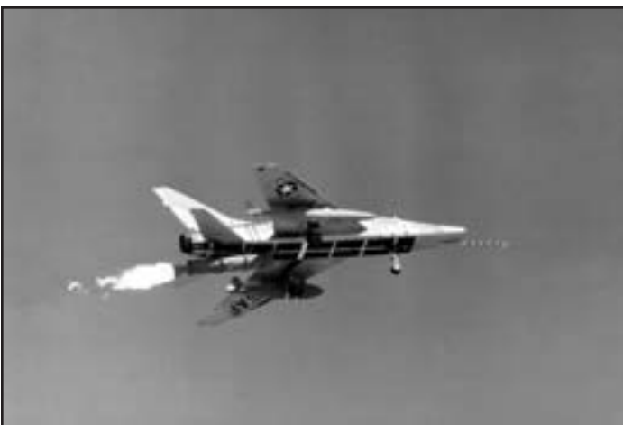
The second ZEL F-100 flight, on 11 April 1958, began with a successful launch. At booster burnout the airplane was traveling 300 mph at an altitude of about 250 feet. Under normal circumstances the booster would separate at this point, but in this case it remained attached to the F-100, making it impossible for the pilot to land safely. (AFFTC History Office)
