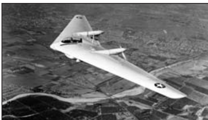
Northrop's N-9M-1 was the first of four subscale flying mock-ups designed to mimic the flying qualities of the XB-35 bomber prototype. The N-9M series provided flight-test data that engineers used to predict the bomber's performance characteristics. (AFFTC History Office)
