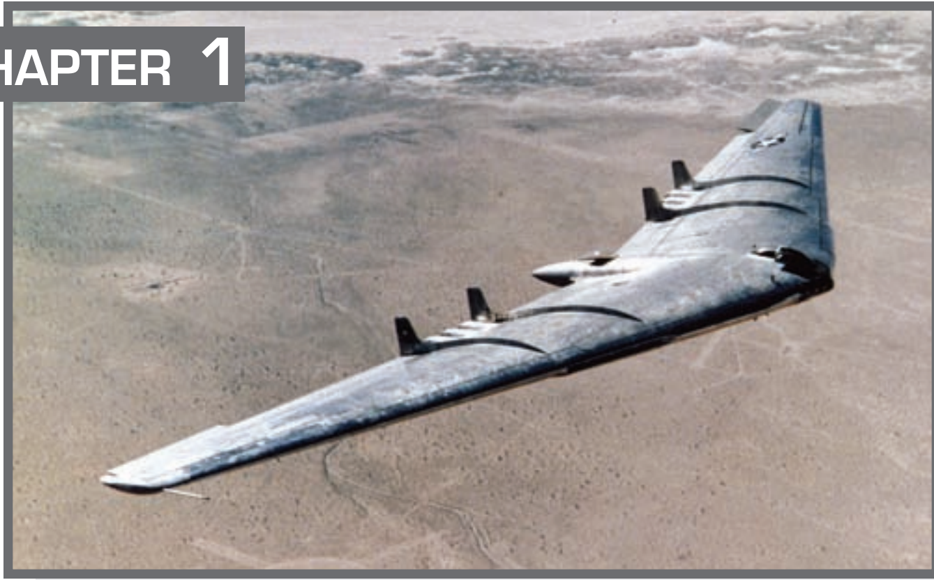
Four prominent vertical stabilizers and wing fences marred the YB-49's clean aerodynamic lines. Test pilots found the flying wing design somewhat unstable as a bombing platform. (AFFTC History Office)
