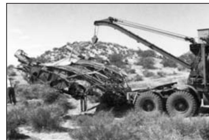
Crash recovery personnel use a mobile crane to remove the cockpit section and engines of the N-9M-1. The remains of the airplane were scrapped following the accident investigation. (AFFTC History Office)
